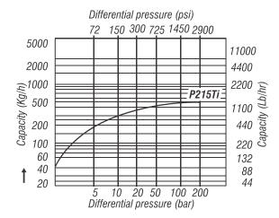
Capacities given are continuous discharge capacities of hot condensate. The cold water capacity at start-up condition will be 2.5 of the hot condensate capacity.
