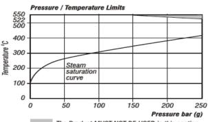
The Product MUST NOT BE USED in this section Note: If the product is used at pressures above 170 bar then a reduction in working life may be experienced.
