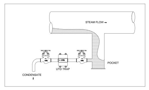
• Testing of trap: trap can be tested either by Test Valve, pyrometer, ultrasonic stethoscope or a rod with sufficient length can be touched to the trap body & vibrations can be sensed by hands if trap is operating.
